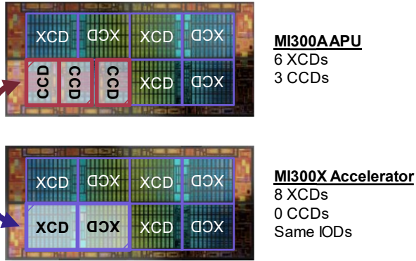
Figure 16. Modular replacement of MI300A’s CCDs with XCDs to create the MI300X accelerator.
