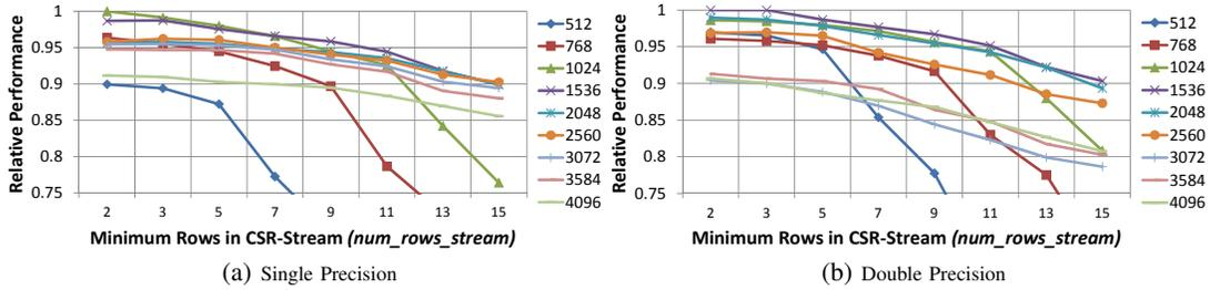
Figure 4. Relative performance of CSR-Adaptive at varying minimum rows in CSR-Stream for a range of NNZ\_PER\_WG. The legend depicts the value of NNZ\_PER\_WG. The values plotted are the harmonic mean of the performance achieved with over 48 different sparse matrices.
