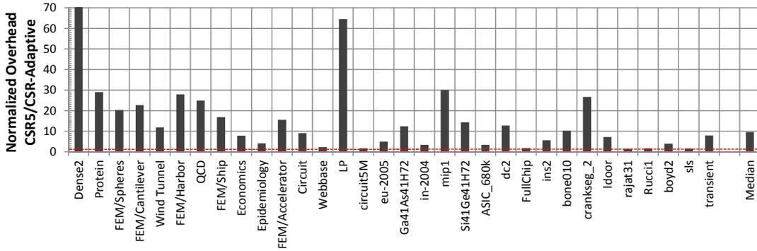
Figure 12. Overhead incurred for generation of specialized data structures in CSR5 and CSR-Adaptive, normalized to CSR-Adaptive (red line)
