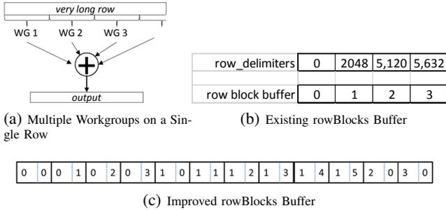
Figure 5. Illustration of multiple workgroups working on a single long row. Three rows contain 2048, 3072, and 512 non-zeros, respectively. The NNZ\_PER\_WG is assumed to be 512 for both existing and improved rowBlocks buffers. In the improved rowBlocks buffer, each entry consists of row and workgroup numbers for workgroups working on that row.
