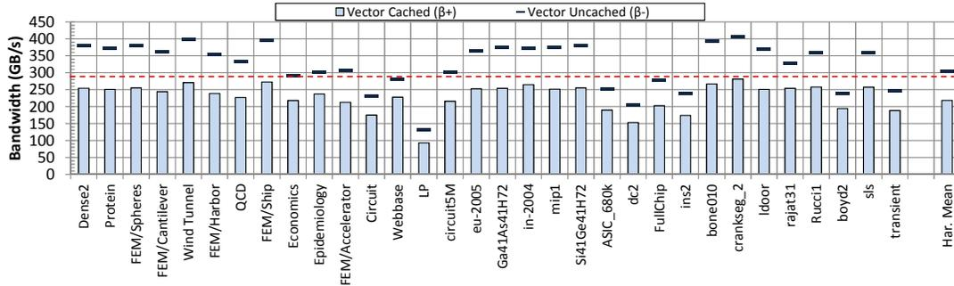
Figure 14. Bandwidth achieved by CSR-Adaptive assuming the vector is either fully cached or uncached. The red dashed line indicates the bandwidth achieved using a STREAM-style microbenchmark. Results are from single precision tests; double precision bandwidth is roughly the same.
