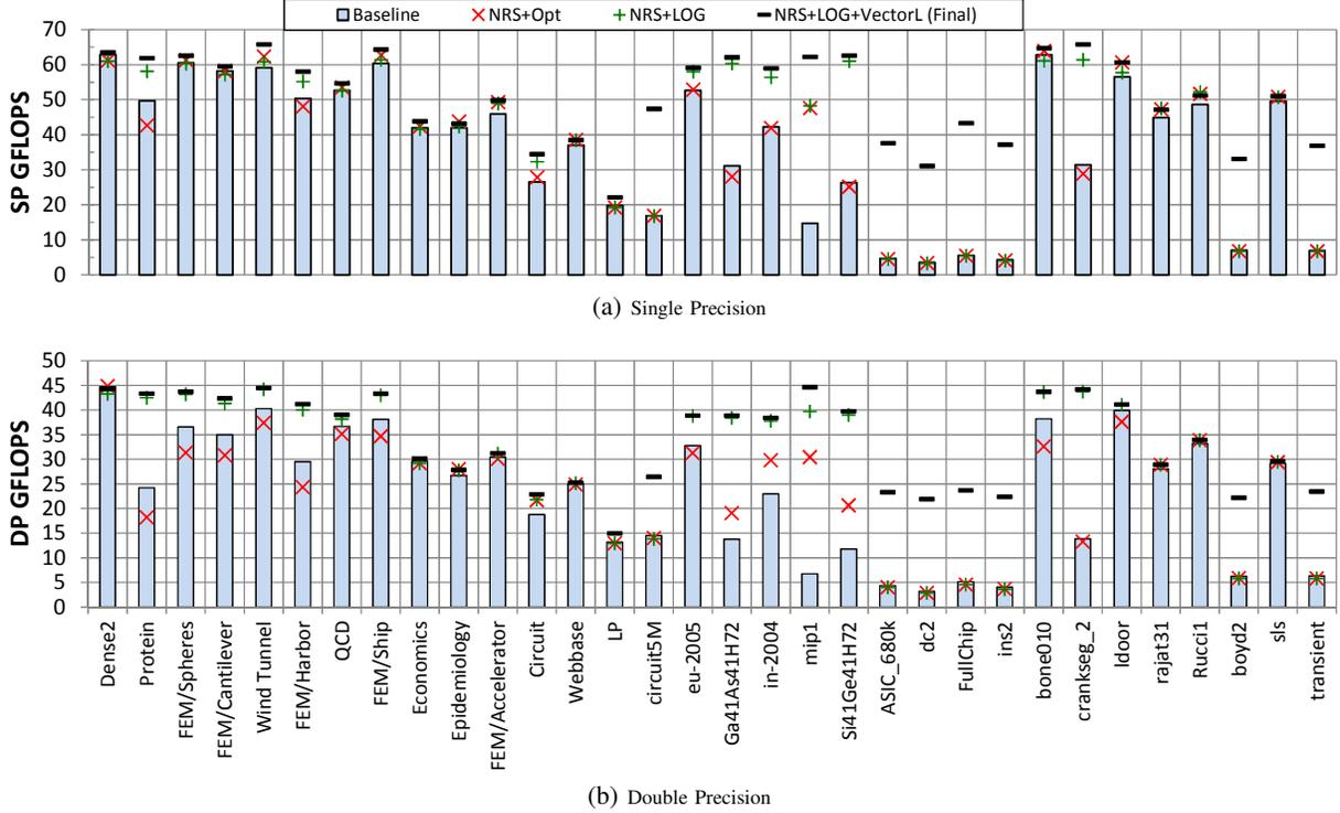
Figure 10. Effect of various optimizations in CSR-Adaptive. NRS: num\_rows\_stream, denotes the performance achieved by optimally choosing the minimum number of rows needed in a row block before using the CSR-Stream algorithm. LOG: logarithmic reductions in CSR-Stream. NRS+LOG denotes the performance achieved by combining NRS and LOG. Lastly, the optimized version combines NRS, LOG, and CSR-VectorL.
