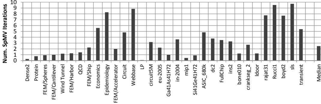
Figure 13. Number of SpMV iterations required to amortize the cost of generation of the rowBlocks buffer using a single CPU core.
